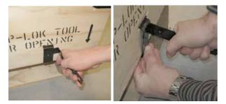
Place the tool behind the clip. Use your other hand to keep the clip in place when you unlock it. Otherwise the clip may cause damage when it springs out of grip.
