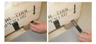
Pull out the Clip-Lok opening tool by using two fingers.
