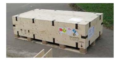
During moving and handling, do not tilt the boxes more than 90 degrees. It might be best to unpack the system outside the building in which the installation is to be made.
