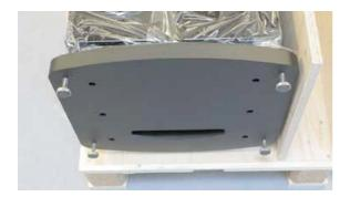
Spikes are the most stable option but might cause damage to the floor below; therefore, the use of spikes will be each customer's own responsibility. Steinway Lyngdorf cannot take any responsibility for any damages caused by spikes. Choose the non-penetrable feet if there are any concerns about potential harm to floors.
