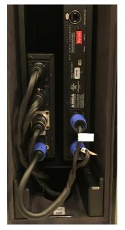
An Model A1 amplifier is powering the Model C speaker. The amplifier is mounted together with the crossover for the mid-high section in a chassis, which is fixed to the top of the box with two M4 screws.
